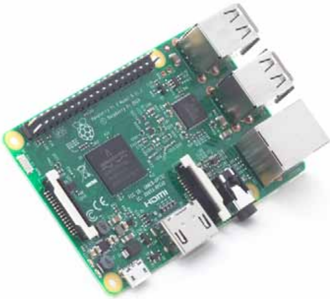
Figure 3 – Raspberry Pi 3 (taken from www.raspberrypi.org )
